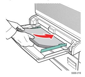
■ Insert Small US postcards **short-edge feed** and **facedown** into Tray 1 (MPT) only. Place the **top** of the postcard toward the **rear** of the printer.
